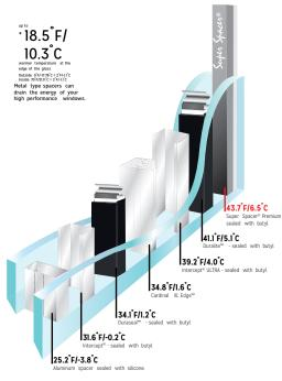
Simulations performed by Enermodal Engineering Ltd. using Window 5.2 and Therm 5.2 as per NFRC100-2001. Outside temperature 0° F, inside temperature 70° F. Low-e glass Cardinal Low-e' 272. Air spaces 500° wide, 90% argon file (IGUS 24° x 48° ID research year) used intercept "was 0.305° thick. Super Spaces", Duralist" and Durassal" are registered trademarks of Quantes Building Products, Intercept is a
